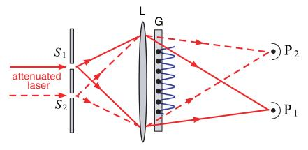
**Figure 1.** Simplified representation of Afshar's experiment [28, 29]. An attenuated laser illuminates a Young's double-pinhole interferometer. A lens (L) images each pinhole  $S_1$  and  $S_2$  on two detectors  $P_1$  and  $P_2$ . A grid of thin wires (G) with a period matching the interfringe is positioned after the lens so that the wires of the grid are exactly superimposed on the dark fringes of the interference pattern.
